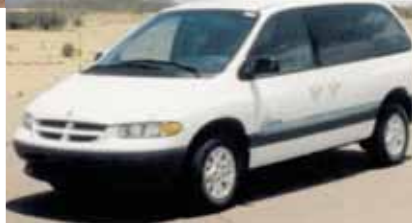
Dodge Caravan electric with NiMH battery
