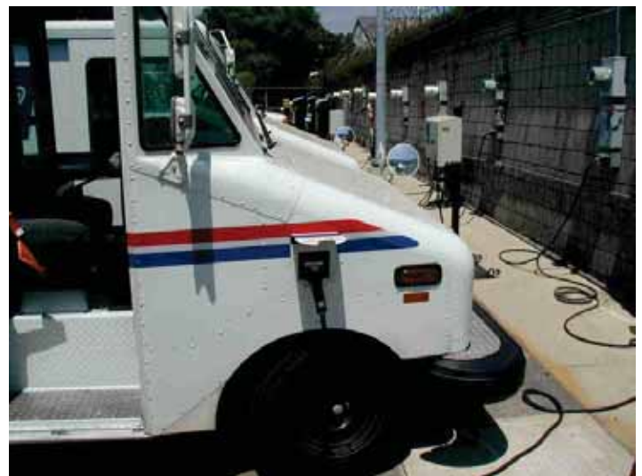
U.S. Postal Service electric carrier route vehicles charging
