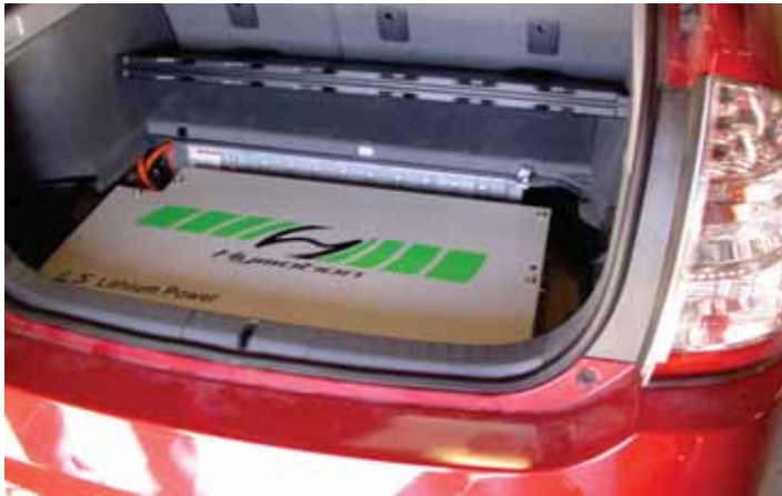
A123 battery installed in the trunk of an A123 Hymotion conversion
